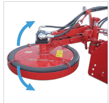
Cutting head can be hydraulically angled using tractor's remote valve to work on slopes and slight terraces
